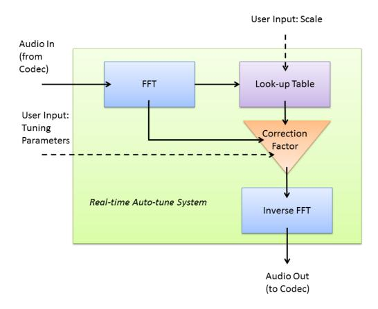
Figure 1: Block diagram of our auto-tune system
