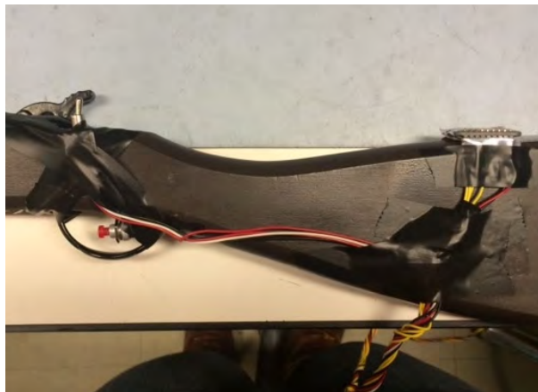
Photo 7. Photo of Rifle Controls Shows "fire" button, "safety" switch, and gyro sensor.
