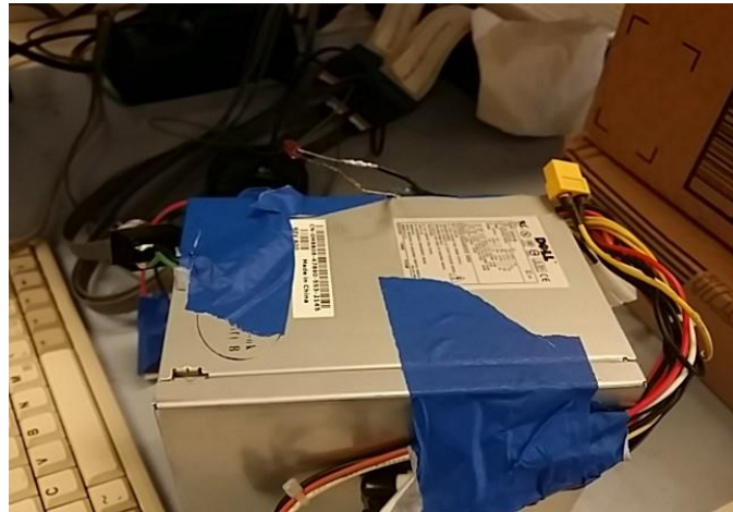
Figure 4: The modified PSU. (From left to right) The switch, led indicator, and female XC60 power connector can be seen in the photo.
