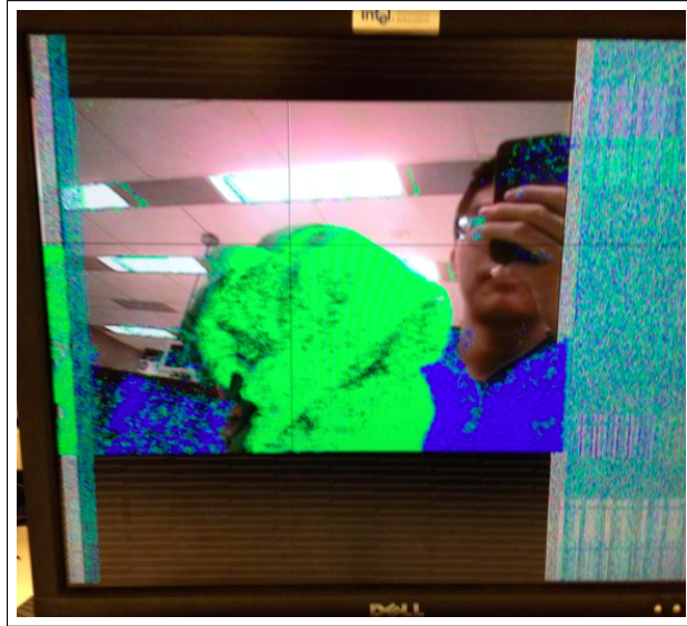
Figure 8: Crosshairs example. Pixels within a range of a target hue were colored over to signal detection. The hue value in the crosshairs was outputted to the hex display for calibration.
