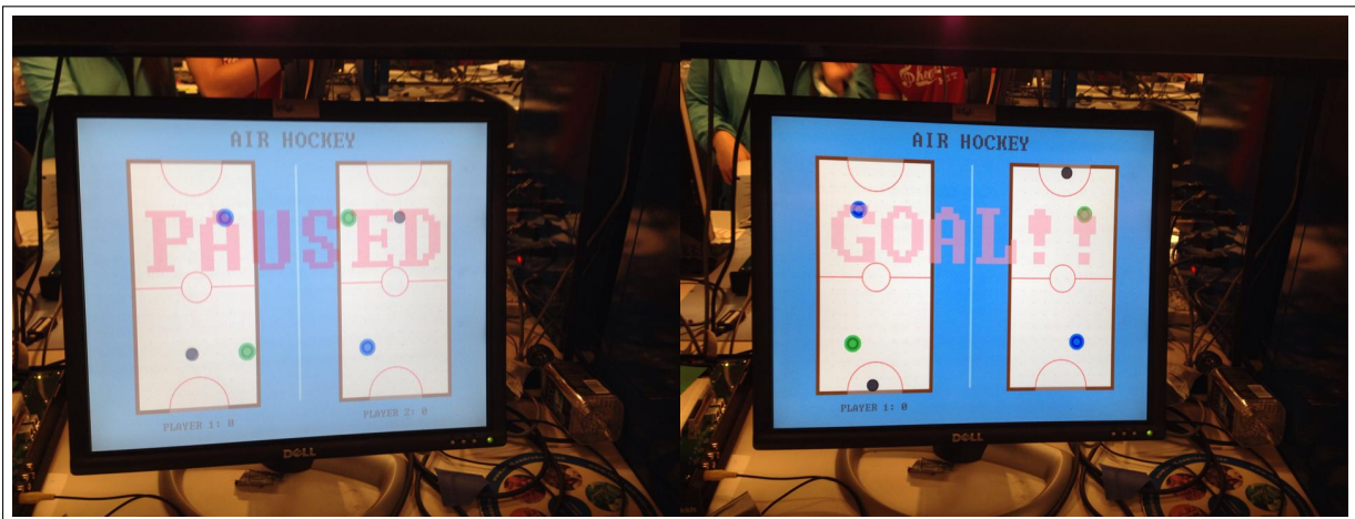
Figure 18: Two examples of the text overlay for the air hockey game. In the left, the player score flashes when a goal is scored. On the right, when the game is paused, the rest of the screen is alpha-blended with a white rectangle.
