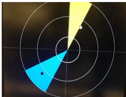
Figure 22. Still moment in color piano demonstration. This displays the combined pixels outputted by the piano logic combined with geometry, alpha blending, and tracking modules.
