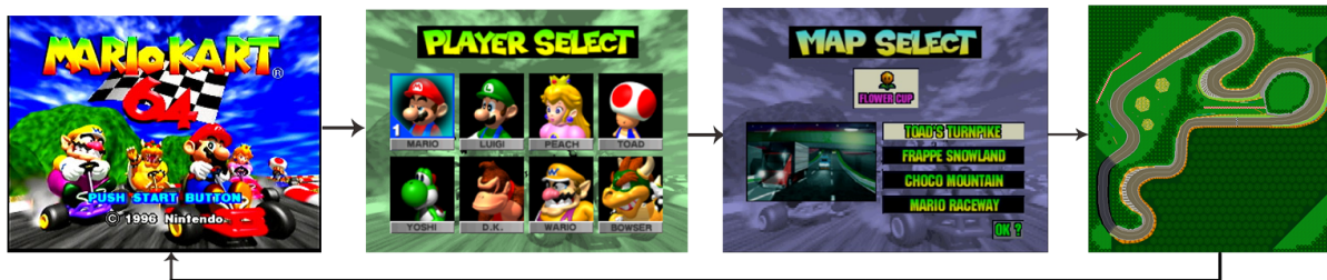
Figure 2: On startup players will navigate through these screens using N64 controllers. The splash screen will transition to the player select screen when a player presses the start button. The player select screen transitions to the map select screen and from there to the actual racetrack as players make selections with the joystick and 'A' button.
