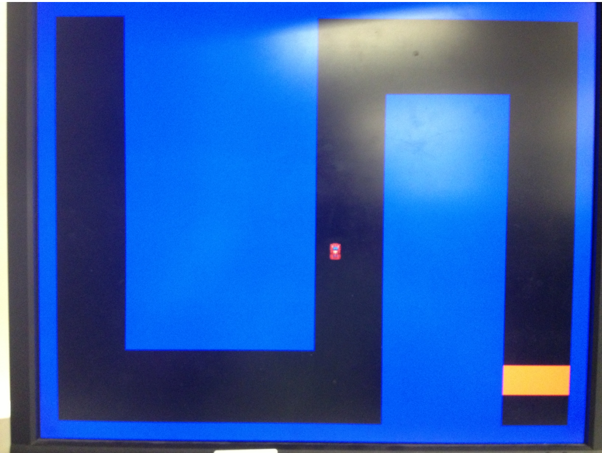
Figure 2: Visualization Module Final Output. This is the display output of the visualization module, containing a car which was to be driven by voice commands in different directions, a maze whose walls the car cannot pass through, and a finish line (here in orange) which will cause the module to display a screen with the word 'DONE' on it upon coming into contact with the car sprite.
