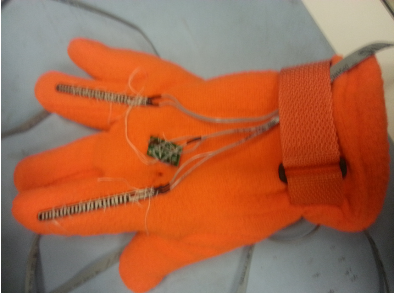
Figure 2: The “Smart Glove” setup. Accelerometer mounted on the glove and flex sensors attached to the ring and index fingers.
