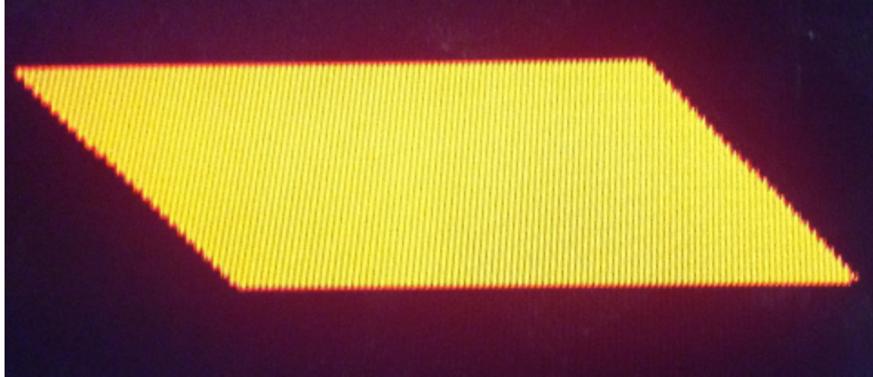
Figure 17: A correctly rendered rhombus. This images shows the results of the renderer, ZBT, and VGA modules when supplied with a polygon with coordinates (50, 50), (200, 50), (250, 100), (100,100).
