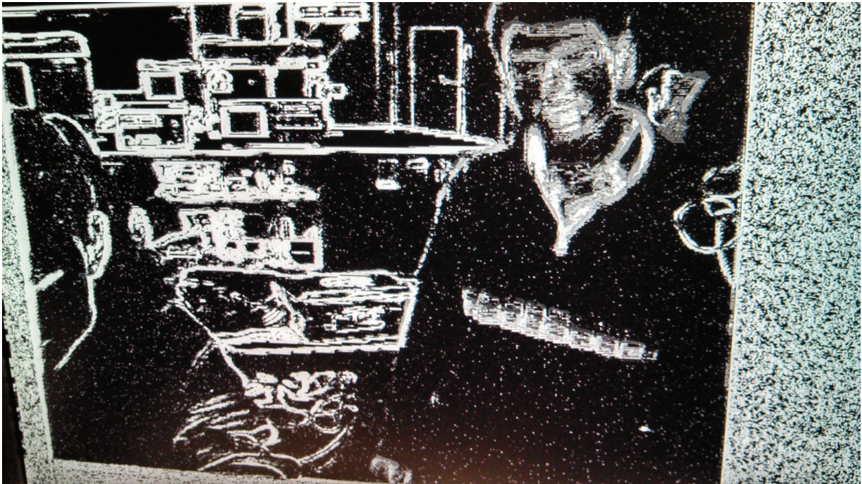
Figure 10: 5x5 Sobel Edge Detection Output
