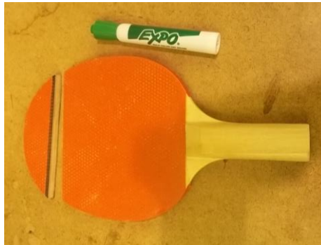
Figure 6: The paddle post-sawing. The paddle was cut along the front edge to provide a flat area that would be more easily be detectable.
