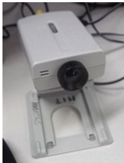
Figure 7: The camera used for tracking the paddle. It was helpful to make the image out of focus in order to avoid identifying the bright blue, pink, and yellow in the background.
