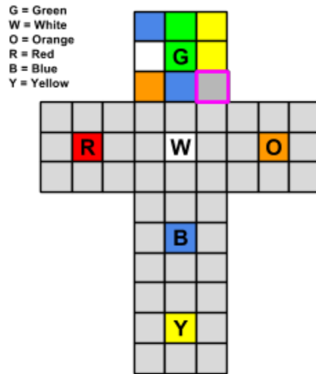
Figure 7 - Input Initial Configuration Screen. User can navigate between the cubelet faces using the arrow buttons on the labkit (selected face highlighted by pink box outline) and input the desired colour by cycling through the 6 options using the appropriate button.
