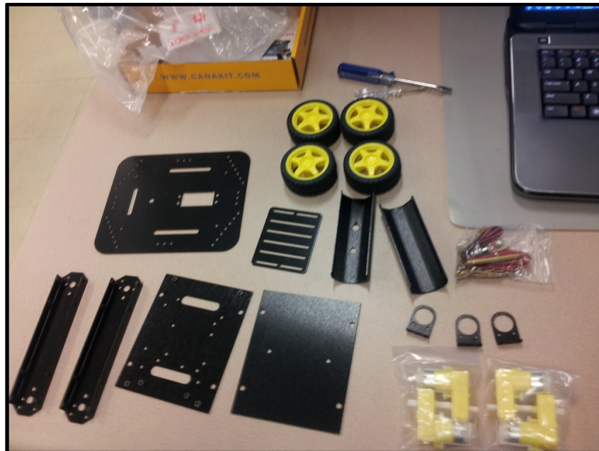
(Figure 5): 4WD Platform before assembly
