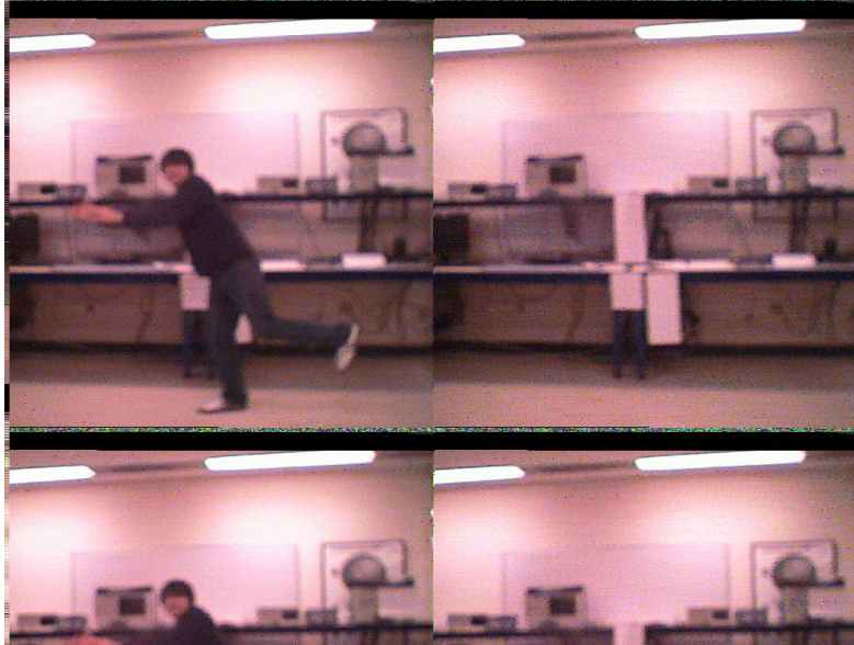
Figure 5 - “Preview” mode shows the 2 banks of ZBT memory, holding the current image (left), along with the reference image (right). Camera is purposefully out of focus to act as a low-pass filter.
