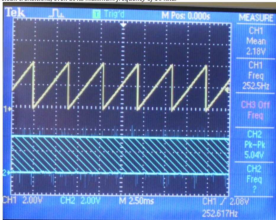
Figure 3: Ramp wave as viewed on oscilloscope. This screenshot is taken from the in-lab oscilloscope and demonstrates a successful ramp (in yellow). Clock_varly is shown in blue, below. The ramp is shown here at its maximum frequency of just above 250 Hz.
