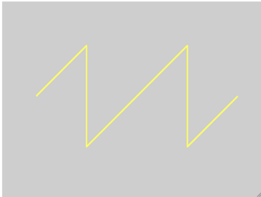
Figure 8: Bitmap image of ramp wave, used on display
