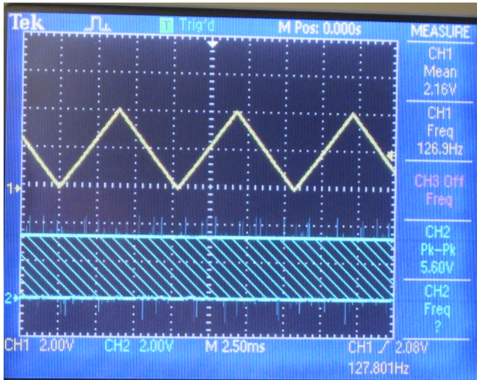
Figure 4: Triangle/sawtooth wave as viewed on oscilloscope. This screenshot is taken from the in-lab oscilloscope and demonstrates a successful triangle (in yellow). Clock_vary is shown in blue, below. The wave is shown here at its maximum frequency of just above 125 Hz.
