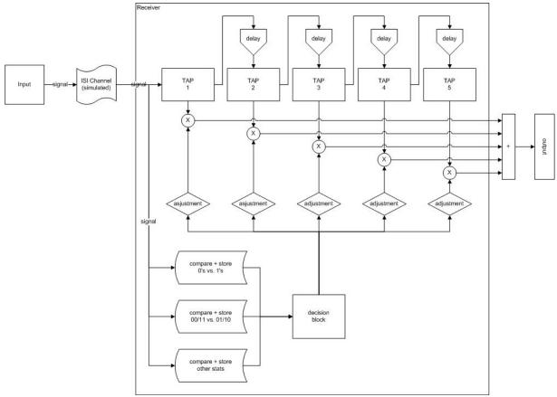
As the signal comes in, the DFE will calculate each tap in turn. Since traditionally a DFE is partly analog and partly digital, our implementation will differ from tradition, since we are using all digital components.
