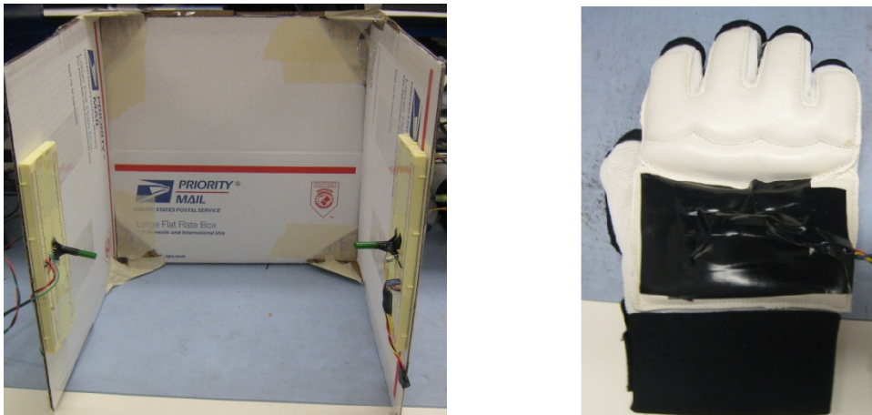
Figure 2. (left to right) IR beam setup and accelerometer chip attached to taekwondo glove
