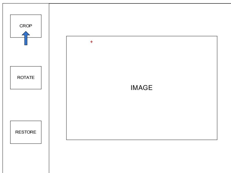
Figure 1. This is what the user will see on the screen. The arrow and plus sign will move in response to movements of the user's left and right fingers, respectively, on the black paper.
