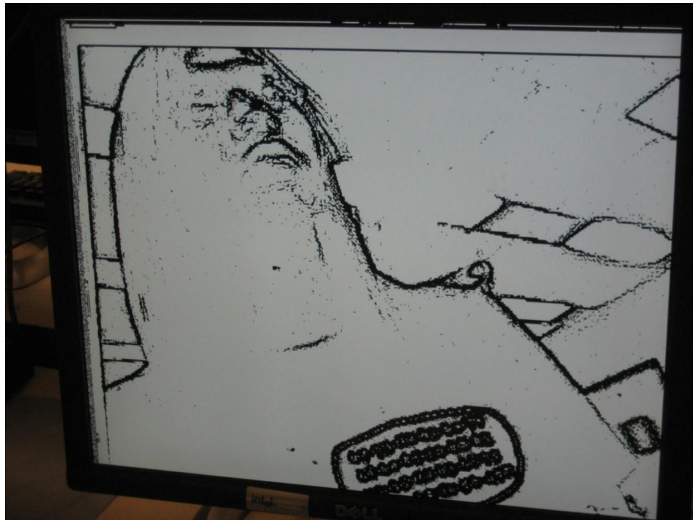
Figure 10: image of Jon that shows the Sobel filter that outputs white for a non-edge and black for an edge
