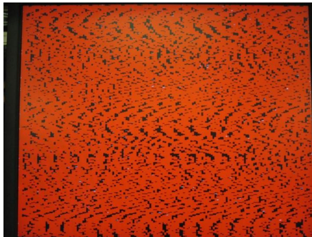
Figure 14: Harris output showing too many "corner" values (pixels in red)
