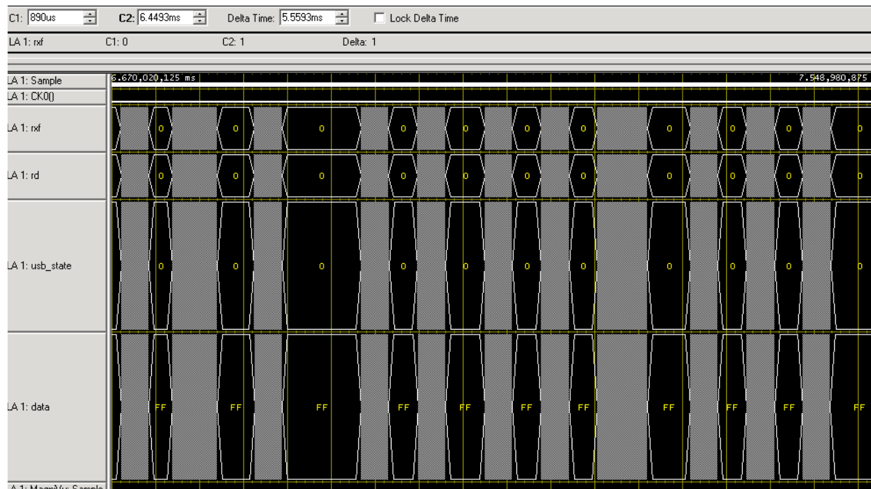
Figure 6: Small gaps in USB transmission of the initial reader state machine
