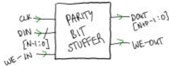
Figure 13: Inputs and Outputs for the Parity Bit Stuffer
