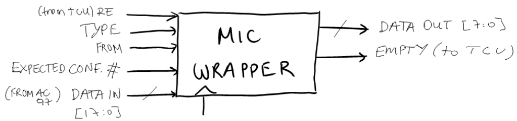
Figure 8 - Block Diagram of the Mic Wrapper showing the inputs and outputs
