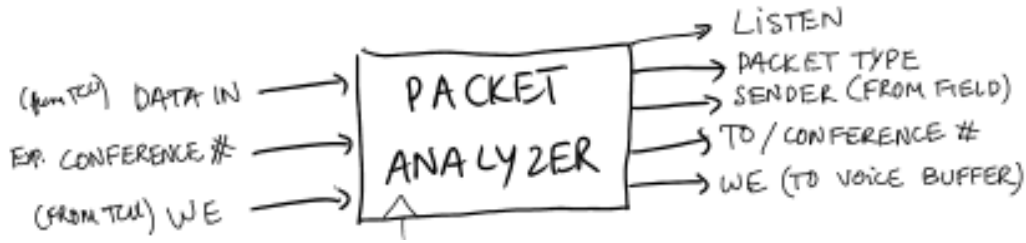
Figure 17: Inputs and Outputs for the Packet Analyzer
