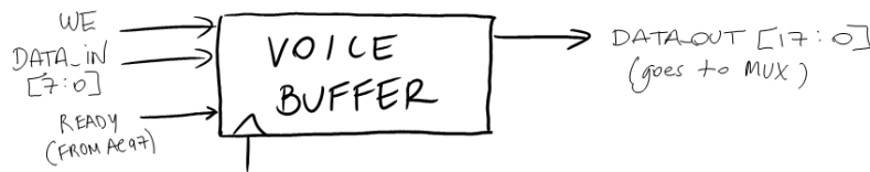
Figure 10 - Block diagram of the Voice Buffer illustrating inputs and outputs
