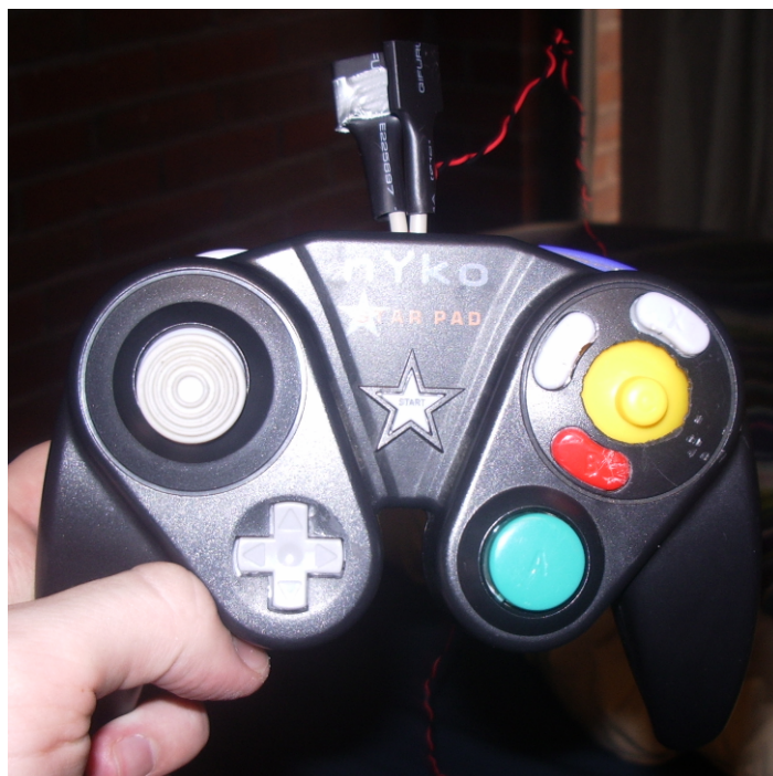
Figure 4: Modified Nintendo Gamecube controller, with new joysticks and working rumble
