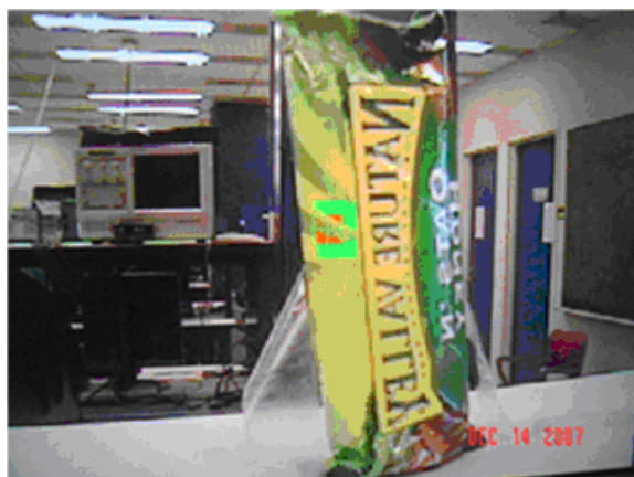
Figure 17: Screenshot of XVGA display, incorporating the pointer detection. Note: the red pixels are used to determine if the pointer is at sight. In this case, the pixel concentration was not high enough, so the module interprets the pixel as “lost.”
