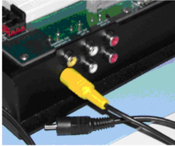
Figure 8: Video input connection to FPGA (taken from ://web.mit.edu/6.111/www/f2006/projects/jburnham_Project_Final_Report.pdf ).
