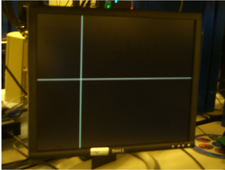
Figure 1. Video Output: The crosshairs on the computer screen show the location of the object.
