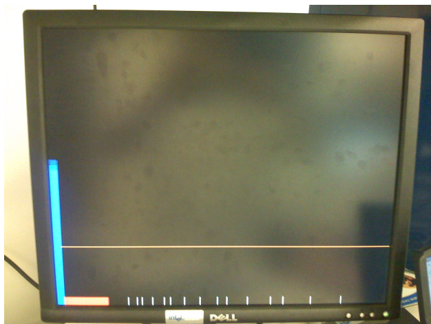
Figure 2.6: A horizontal line, orange in color, is displayed near the bottom of the screen in response to a low frequency with sufficient magnitude.
