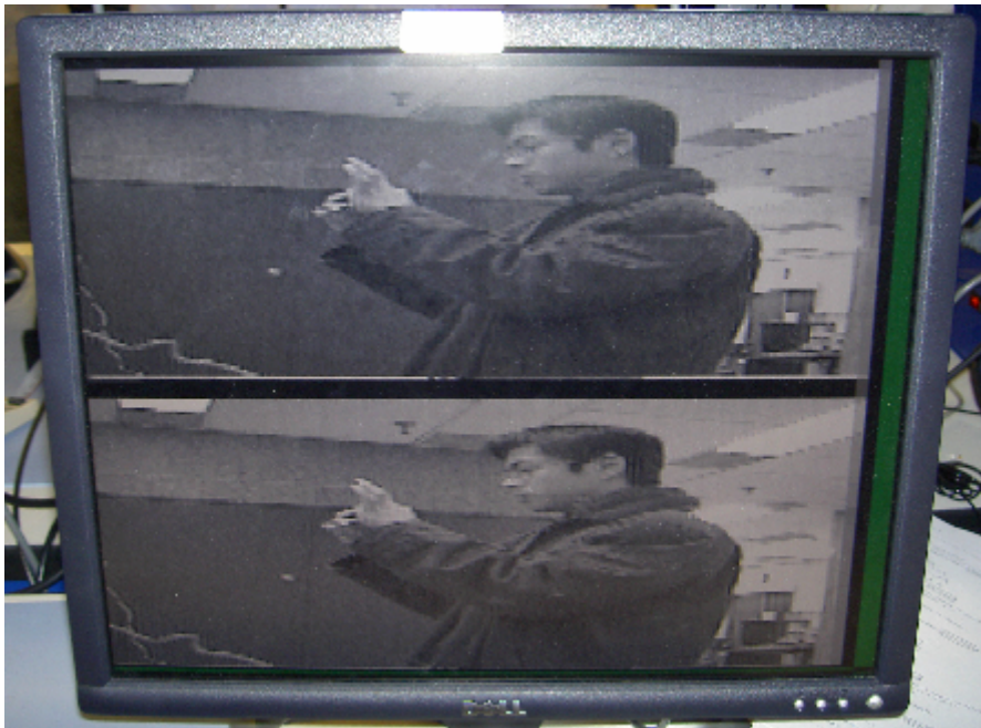
Figure 8: Luminance data from memory A (top picture display) and B (bottom picture display) are shown above on the monitor. The two displays are a constant frame length apart in order to allow for motion detection to capture slower movement.
