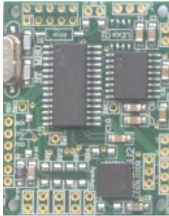
Figure 2: Accelerometer chip LIS3L02DQ 3axis digital output The evaluation board came with power regulations and standard output pins
