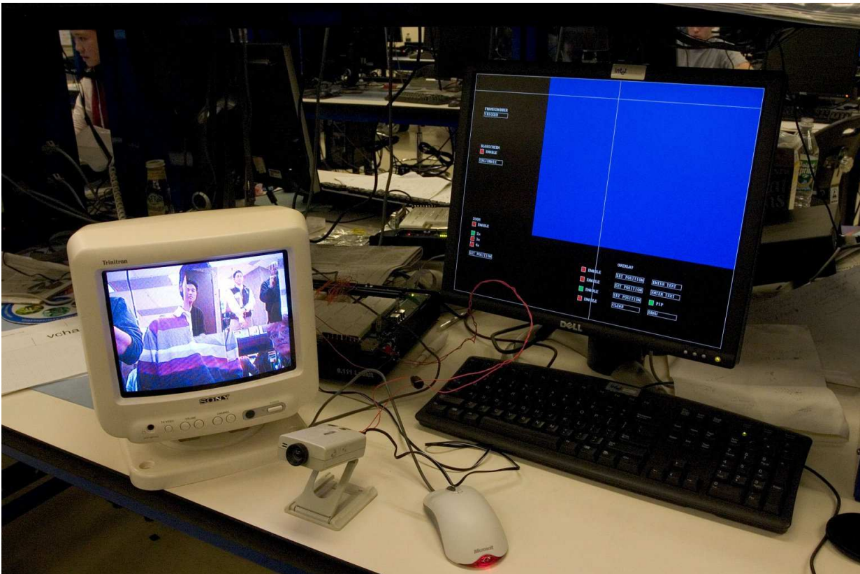
Figure 1: Video Effects Processor in Operation - The flat panel monitor shows the user interface used to control the system. The television on the left shows a sample output - note the picture-in-picture window in the corner of the screen.
