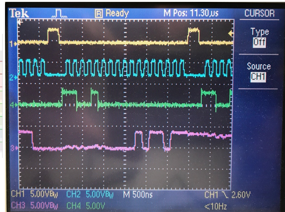
Oscilloscope Analog Capture of different SPI transaction
