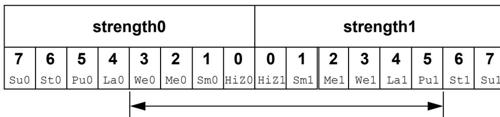
Figure 28-10—Range of strengths for an unknown signal
