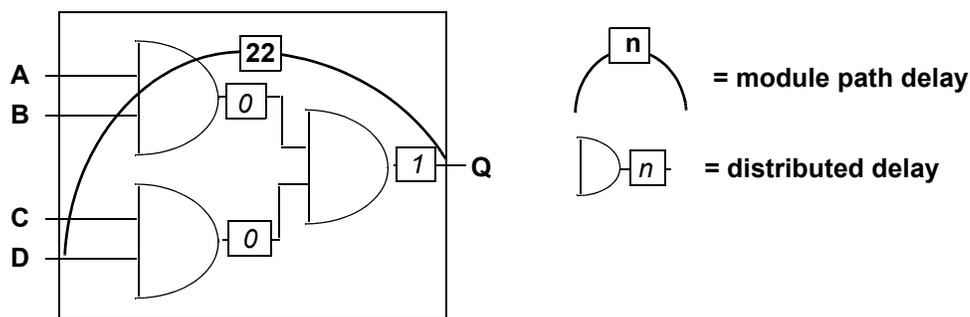
**Figure 30-3—Module path delays longer than distributed delays**
