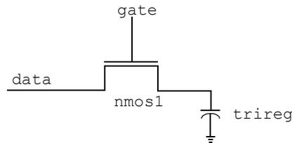
**Figure 28-26—Trireg net with capacitance**
