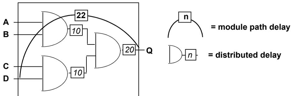
Figure 30-4—Module path delays shorter than distributed delays
