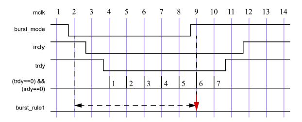
Figure 16-12—Match with throughout restriction fails
