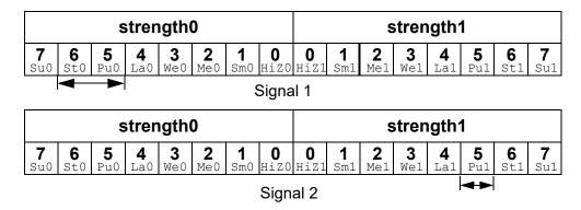
The combinations of strength levels for and logic appear in the following chart:
