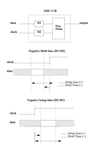
Figure 31-5—Data constraint interval, negative setup/hold
