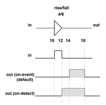
Figure 30-6—On-detect versus on-event
