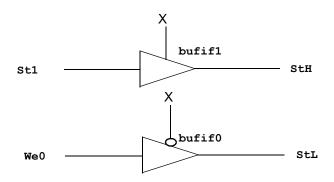
Figure 28-6—Bufifs with control inputs of x
