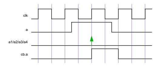
Figure 16-17—Clocking blocks and concurrent assertion
