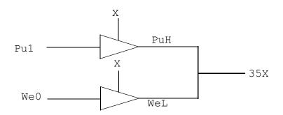
Figure 28-9—Combined signals of ambiguous strength
