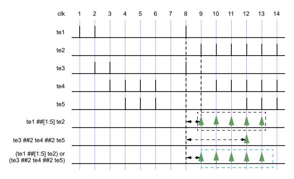
Figure 16-11—ORing (or) two sequences, including a time range
