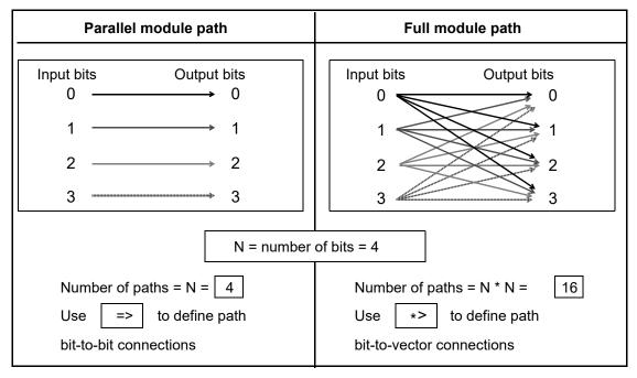
Figure 30-2—Difference between parallel and full connection paths
