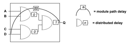
Figure 30-3—Module path delays longer than distributed delays
