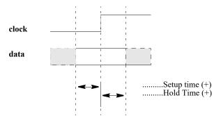
Figure 31-4—Data constraint interval, positive setup/hold
