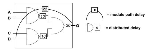
Figure 30-4—Module path delays shorter than distributed delays
