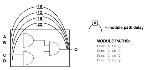
Figure 30-1—Module path delays
