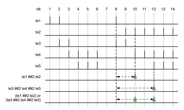
Figure 16-10—ORing (or) two sequences
