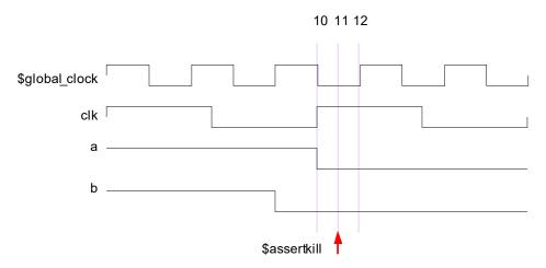
Figure 39-1—Assertions with global clocking future sampled value functions
