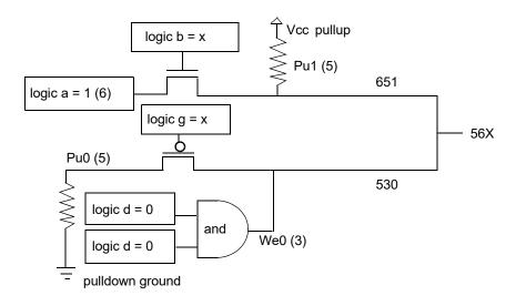
Figure 28-11—Ambiguous strengths from switch networks
