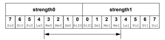
Figure 28-5—Weak x signal strength
