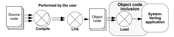
Figure J.1—Inclusion of object code into a SystemVerilog application
