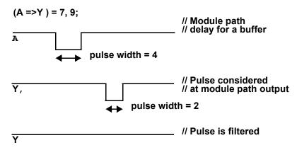
Figure 30-5—Example of pulse filtering
