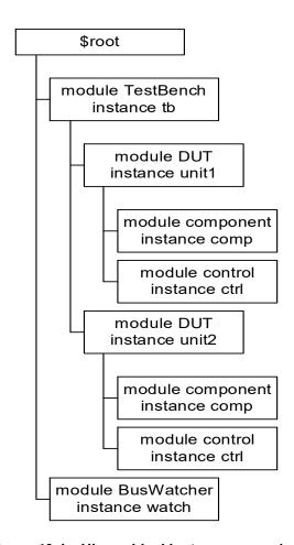
Figure 40-1—Hierarchical instance example
