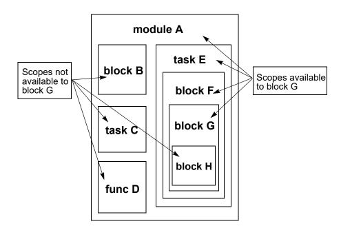
Figure 23-2—Scopes available to upward name referencing
