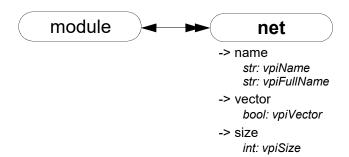
Figure 37-1—Example of object relationships diagram
