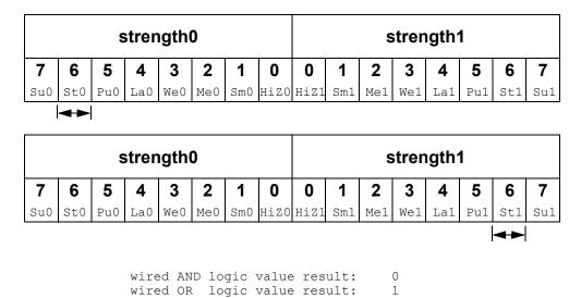
Figure 28-24—Wired logic with unambiguous strength signals
