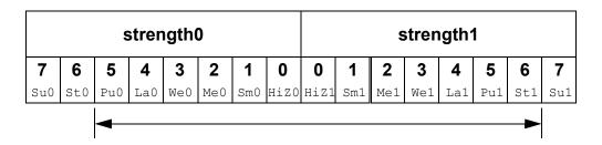
Figure 28-14—Unknown value with a range of strengths
